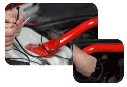
Pull the 3-pin connector and and grounding cable to the front of the vehicle, then tuck the three pin cable back for now.
